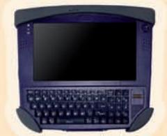
MRC 1100, powerful rugged tablet PC, features 7-inch WVGA TFT LCD with the daylight readable solution and low power processor. Its ergonomic design with a full QWERTY keyboard allows easy operation for mobile workers. More accessible I/O interfaces can be extended via the docking station.
