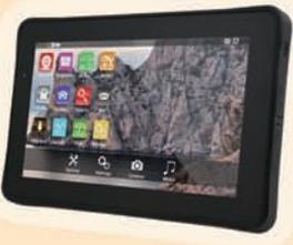
This rugged tablet PC utilizes the Android Operating System to maximize your software options. RTC-700/900 supports high performance and low power consumption NVIDIA® processor. The high capacity battery provides about 12 hours running time for operator usage during the whole working day. The compact size and light weight brings tremendous mobility to any application. The latest design has scratchproof LCD and protection against shock, vibration, water and dust.
