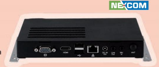
The NDIS B324 powered by the new Intel J1800 processor (formerly codenamed „Bay Trail“) can handle very rich multimedia contents. To allow fast content update, the B324 incorporates the industrial-leading USB 3.0 as standard. Support for a diverse variety of OS options including open resource Linux and Microsoft's Windows®, allows users to select between Windows 7 and even Windows 8.
